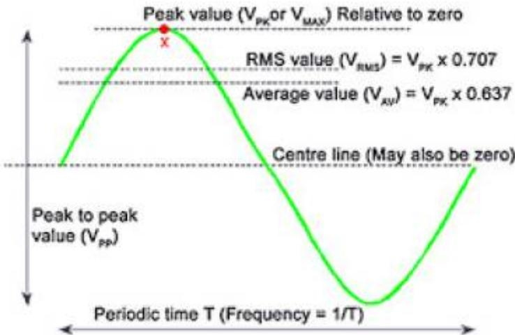
These values can be easily converted to each other. The way formulas for these conversions differ upon the the waveform that applies (sinus, triangle, square). The relevant basic conversions are:
