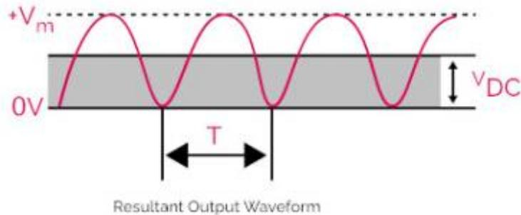
The output voltage of the rectifier is lower +/- 1.4V lower than the input voltage. This is due to the forward-biased (conducting) voltage over two diodes. Due to voltage over the diodes the maximum peak value is:
