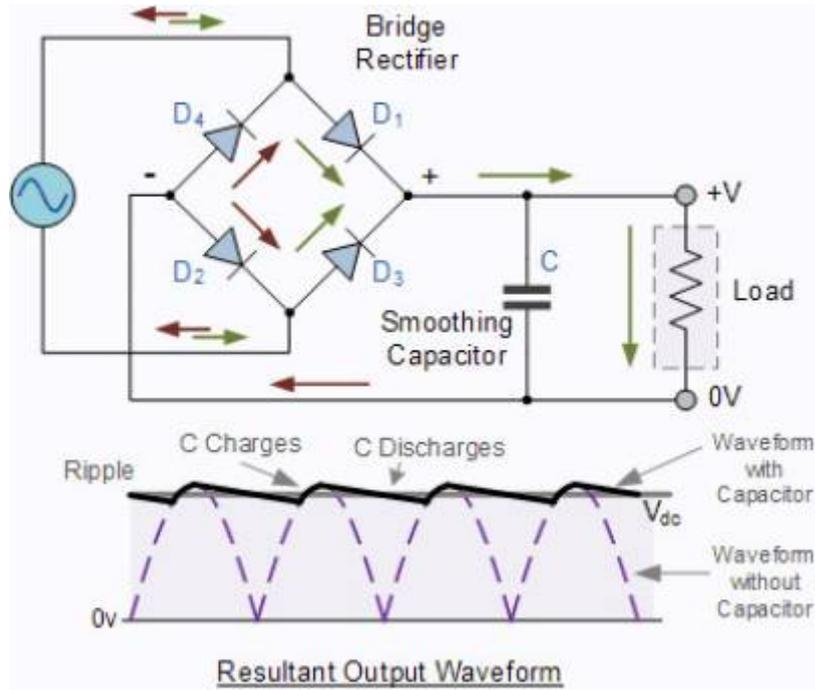
We can improve the average DC output of the rectifier while at the same time reducing the AC variation of the rectified output by using smoothing capacitors to filter the output waveform. Smoothing or reservoir capacitors connected in parallel with the load across the output of the full wave bridge rectifier circuit increases the average DC output level even higher as the capacitor acts like a storage device.
