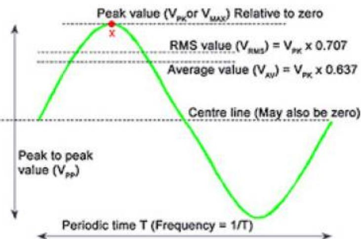
These values can be easily converted to each other. The way formulas for these conversions differ upon the the waveform that applies (sinus, triangle, square). The relevant basic conversions are:
