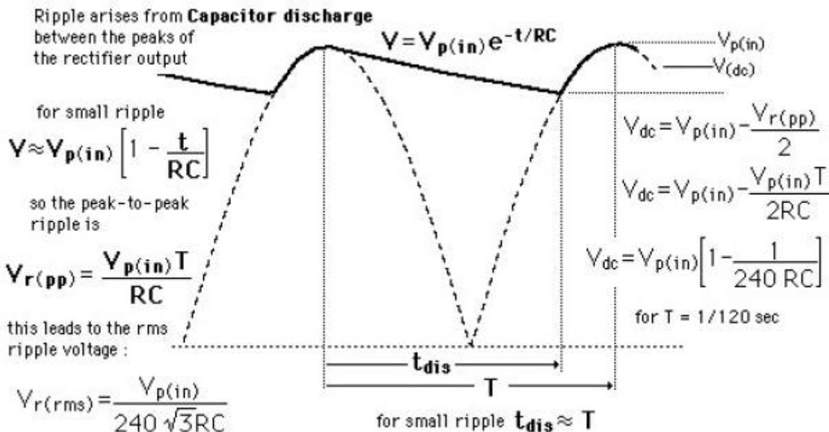
For a full wave rectifier with filter the output voltage can be calculated with the following formula:
