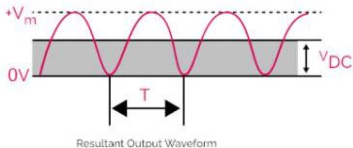
The output voltage of the rectifier is lower +/- 1.4V lower than the input voltage. This is due to the forward-biased (conducting) voltage over two diodes. Due to voltage over the diodes the maximum peak value is:
