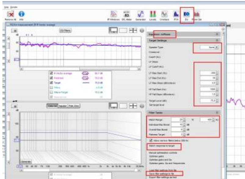
Under Filter tasks hit “Match response to target”. Hit EQ filters button to get dialog for additional manual filter adjustment. Hit Save filter settings to file to save REW EQ filter (use XML format to imported into rePhase).
